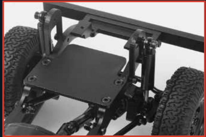
The G2 Chassis features a simple front mounted electronics plate for easy mounting of the XR2 Micro ESC/Receiver combo.
