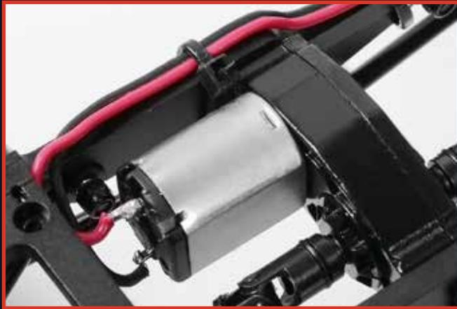
The G2 includes the new Mini Hammer Transfer Case. Packed with scale detail, the Hammer features a cast metal exterior and heavy duty gears for durability.
